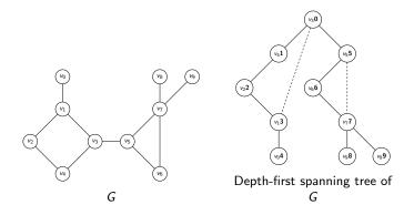
In a Depth-first spanning tree, *depth first number (dfn)* of a vertex v, denoted by dfn(v) is the discovery time of v (shown on the right side of the vertices in bold). Dashed edges are the back edges.
